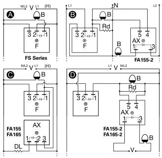
$\begin{array}{ll} V = Voltage & N = Neutral & B = Beacon \\ DL = Dummy Load for Constant Line Loading \\ Rd = 3.3 \ K\Omega @ 5W for 120VAC; 8.5 \ K\Omega @ 5W for 230VAC \\ F = Flasher (FS155-30T, FS155-30RF, FS165-30T) \\ AX = Auxiliary Unit (FA155, FA155-2, FA165, FA156-2) \\ \end{array}$
