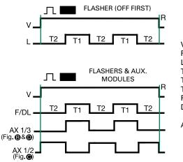
V = Voltage R = Reset L = Load T1 = ON Time T2 = OFF Time T1  $\cong$  T2 F = Flasher DL = Dummy Load AX = Auxillary Module
