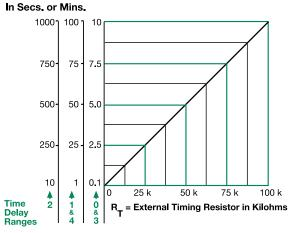
This chart applies to externally adjustable part numbers. The time delay is adjustable over the time delay range selected by varying the resistance across the R⊤ terminals; as the resistance increases the time delay increases
