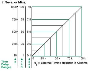
This chart applies to externally adjustable part numbers. The time delay is adjustable over the time delay range selected by varying the resistance across the RT terminals; as the resistance increases the
