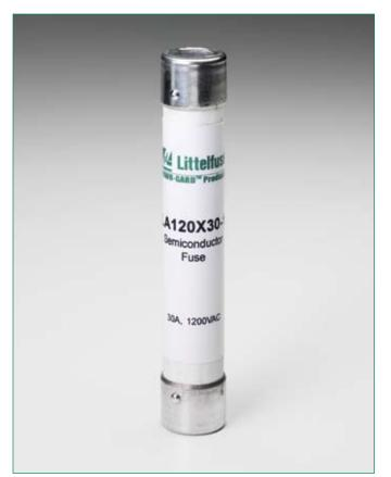
Littelfuse LA120X semiconductor protection fuses, rated ½ through 30A, 1200 VAC are popular for use in traction drive auxiliary circuits and similar applications. LA120X fuses are also suitable for use on 1000VDC auxiliary circuits with low time constants.
